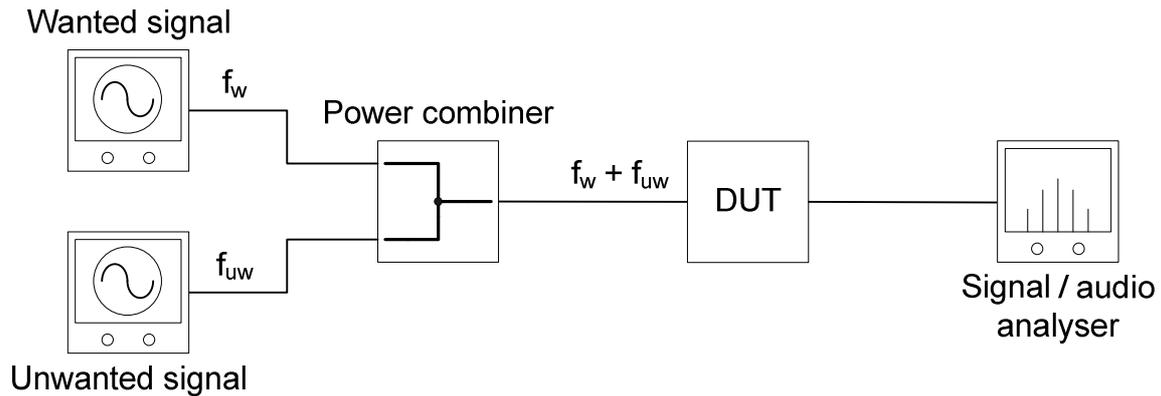
**Figure 6: Measurement setup for receiver adjacent channel selectivity**
