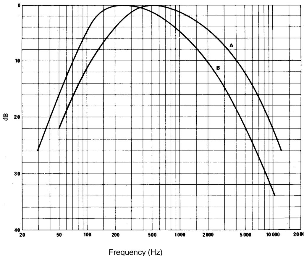
Curve A = Frequency spectrum of standardized noise (measured with one-third octave filters).
