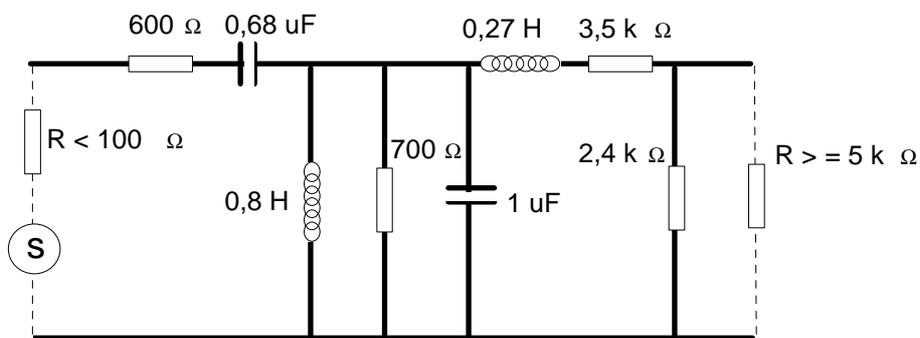
**Figure 2: Filter circuit**
