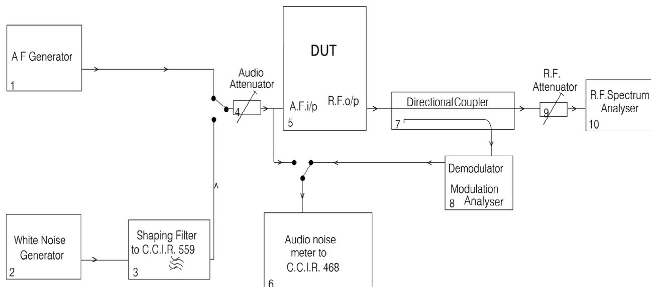
NOTE 1: If the DUT incorporates ancillary coding or signalling channels, for example, pilot tone, etc. these should be switched on prior to measuring the transmitter RF output spectrum.
