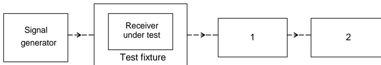
NOTE 1: Coupling device, e.g. AF load/acoustic coupler (in the case of speech equipment).
